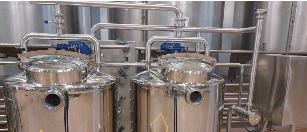
Supplying and fabricating new syrup dissolving unit
